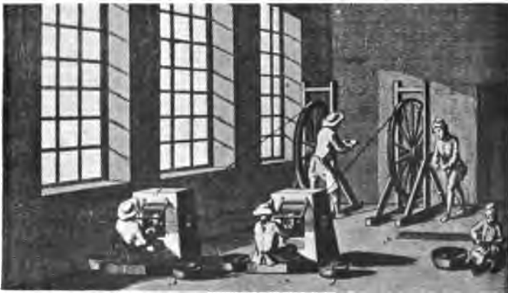
FIG. 65.—Workshop of a Norman Pin-maker (18th century). The Workers are seated before glass Screens, which safeguard the Eyes from Dust and Filings.
